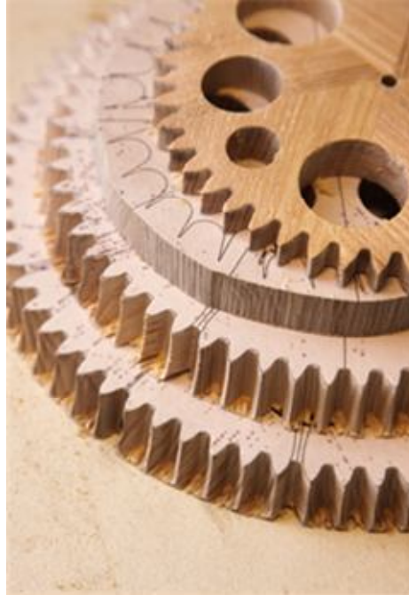
▲...like these. CAD-generated templates are glued to the gear blanks to guide cutting; the weight-saving voids in the finished gear help to reduce starting friction
