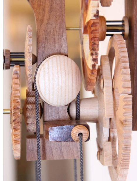
▲ Oil-free: with the judicious use of some modern materials in the pivots, Bruce is able to run his clock without any additional lubricants
