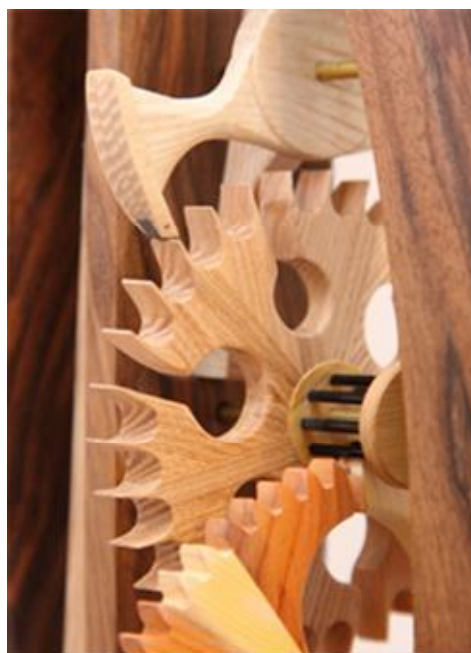
▲ The trundles in the pinion between the escape and intermediate wheel are roller bearings made of carbon fibre tube and 'occultanium'
