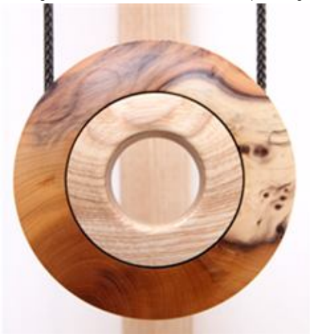
▲ One of the very few bought-in parts in the clock is the ball race in the winder, or counterweight, which allows the turned finger-pull in the centre to spin within the outer turning
