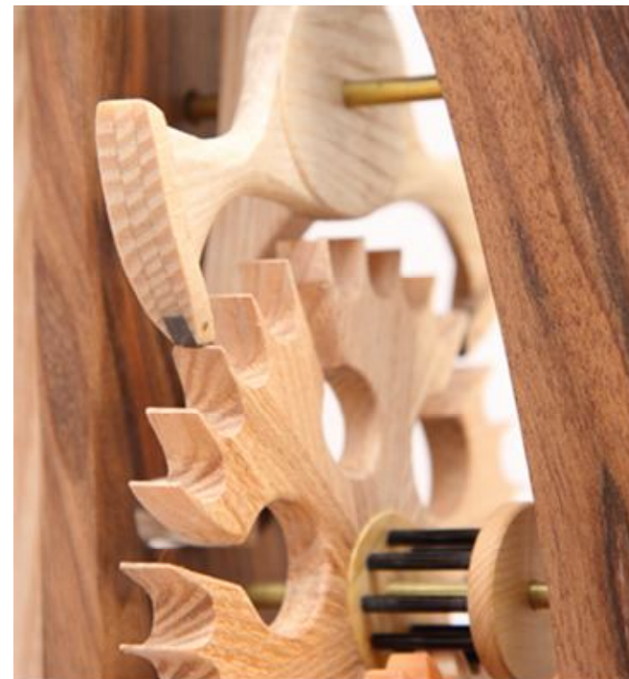
◀ You can see here that the pallets of the escape anchor are laminated so that a PTFE tip can be incorporated between the layers; the escape anchor itself is made in two overlapping parts so that Bruce can adjust their geometry to perfect the contact between the pallets and the teeth of the escape wheel
