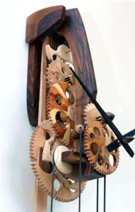
▲ While larger wheels are of segmented construction to keep the grain running radial, the smaller first and second wheels, with their comparatively large and well-spaced teeth, can be made from solid timber
