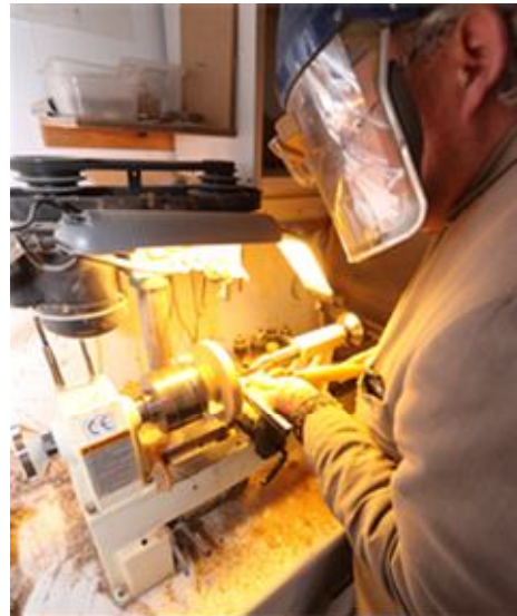
▲ A small Axminster woodturning lathe can also be adapted for cutting gears...
